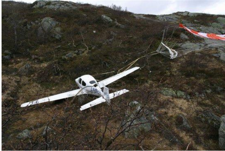
Closer view of same accident site showing aircraft and deployed parachute
