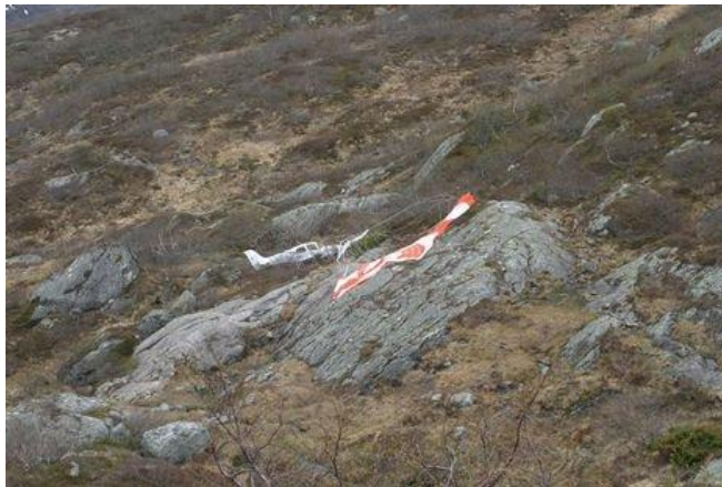
Cirrus SR-20 after deploying its on-board BRS-supplied emergency parachute system
